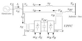
Fig 1: Heffron-Philips model of a power system installed with UPFC
