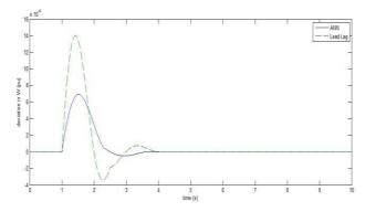
Fig 3: Angular velocity deviation during step change in mechanical input power for nominal load (mb Controller)
